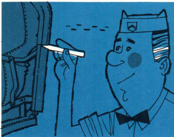
Header bow adjustment
