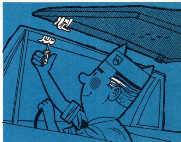
Dowel pin alignment
