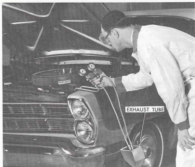
Fig. 29 — Discharging the Refrigerant
