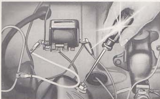
Fig. 22 Checking Overdrive Circuit—Voltage
